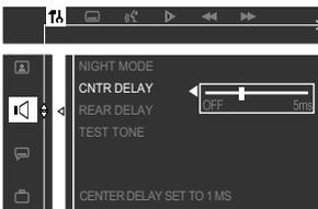
{CNTR DELAY} – Select this to set the delay time in relation to the listening position/distance from the center speaker (5ms, 3ms, 2ms, 1ms or OFF.)
