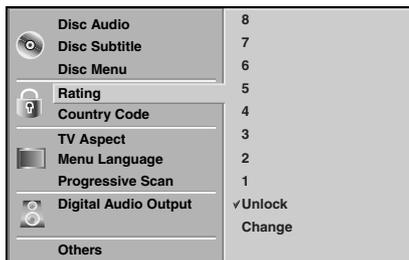
**1** Select "Rating" on the Setup menu using the ▲▼ buttons.
