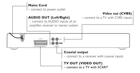
Caution: Do not touch the inner pins of the sockets on the rear panel. Electrostatic discharge may cause permanent damage to the unit.
