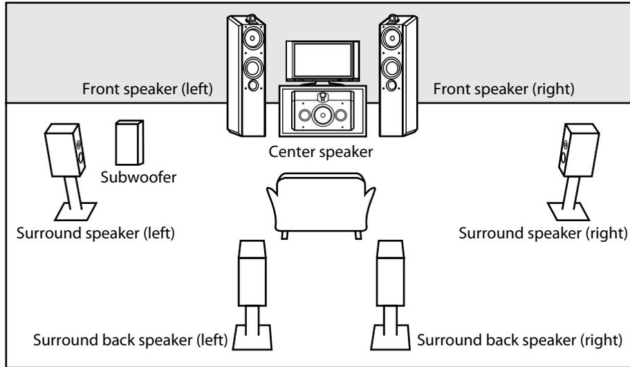
To make the most of its feature, set up your speakers appropriately by referring to the table below.
