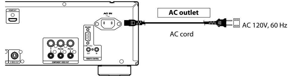
**Supplied cables used in this connection are as follows:**
