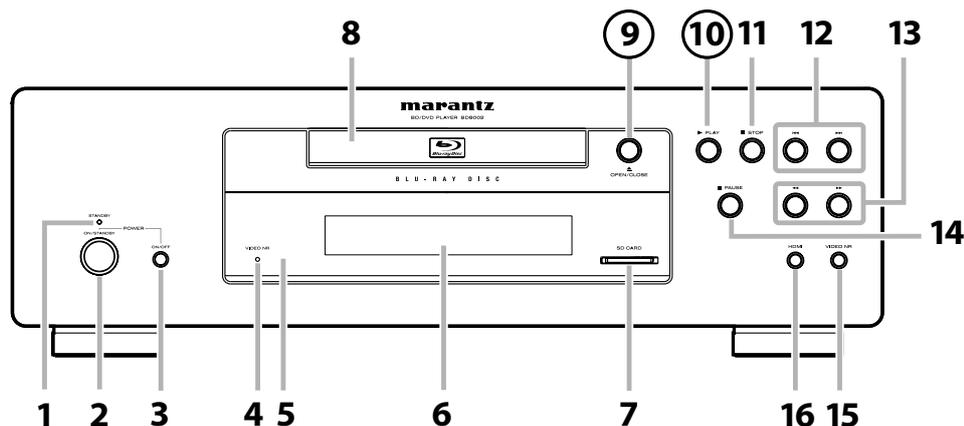
The unit can also be turned on by pressing the buttons with circled numbers.
