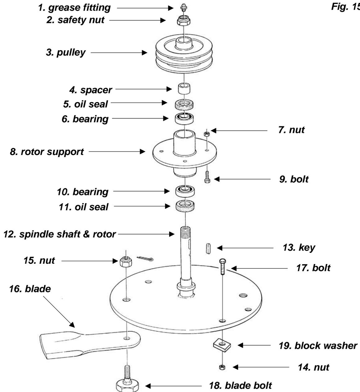
To reassemble the blade spindle, do the following:
