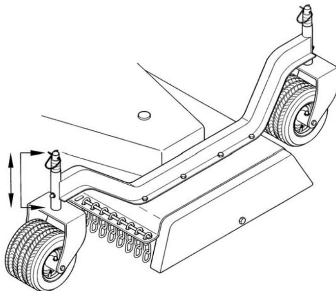
The cutting height is the distance from the blades to the ground. The cutting height is adjusted by **moving the spacers on the wheel yokes**. Placing spacers between the wheel arm and the wheel yoke raises the cutting height by the size of the spacer. Removing the spacers lowers it by the same height (see fig. 5).
