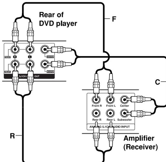
**Analog connection to a multi-channel A/V receiver with 6 Channel connectors (Dolby Digital, DTS):** This DVD Player contains a multi-channel decoder. This enables playback of DVDs recorded in Multi-channel Surround without the need for an optional decoder.
