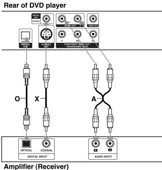
**Amplifier equipped with 2-channel analog stereo or Dolby Pro Logic II / Pro Logic:** Connect the left and right AUDIO OUT jacks on the DVD Player to the audio left and right IN jacks on your Amplifier, Receiver, or Stereo System, using the audio cables (A).
