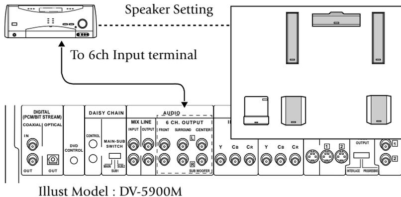
**Setup for 6-channel audio connection:**
