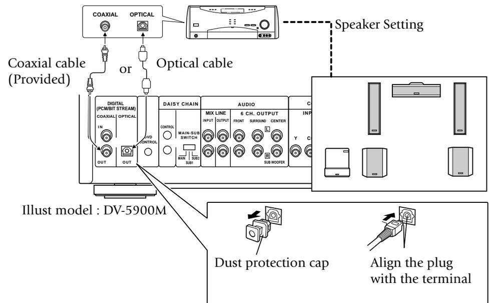
**Note : When connecting the optical digital audio cable**
