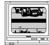
Picture turbulence due to sync unmatching.
