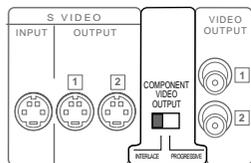
Select the scanning method of the Component Video output using the **COMPONENT VIDEO OUTPUT** switch on the rear panel.
