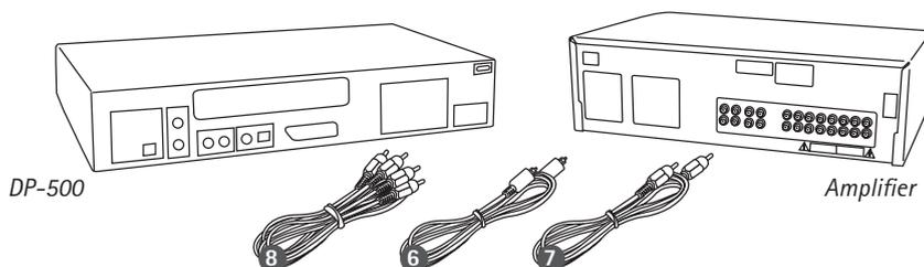
Connecting your KiSS DP-500 DVD player to your amplifier can be done with any of the cables below. (Only one cable can be connected at a time).
