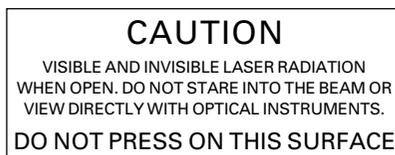
Inside this laser product, a laser diode classified as Class 2 laser radiation is contained as alerted by the internal caution label shown above. Do not stare into beam or view directly with optical instruments.
