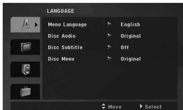
2. Use ▲ / ▼ to select the desired option then press ▶ to move to the second level. The screen shows the current setting for the selected item, as well as alternate setting(s).
