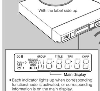
Each indicator lights up when corresponding function/mode is activated, or corresponding information is on the main display.
