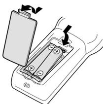
The batteries will last about six months with normal use. If the functions of the remote control become erratic, replace the batteries.
