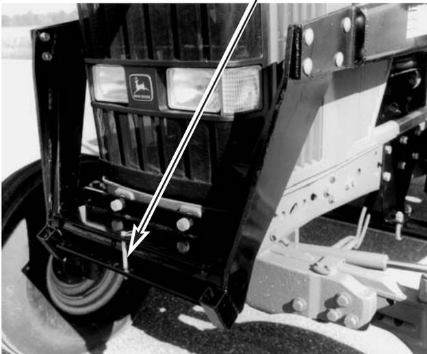
F. Extend bucket cylinder (dump) until subframe rest on rear bracket.
