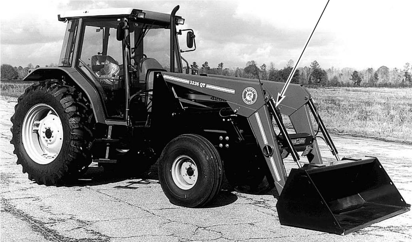
J. Secure hydraulic hoses to tractor to prevent interference. It is recommended that hoses be routed under tractor operator's platform.
