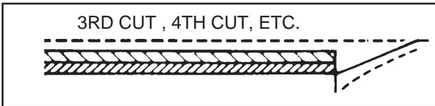
Make additional passes until the desired depth is reached. During each pass, only use the bucket control while at working depth. This will allow you to concentrate on controlling the bucket angle to maintain a precise cut.
