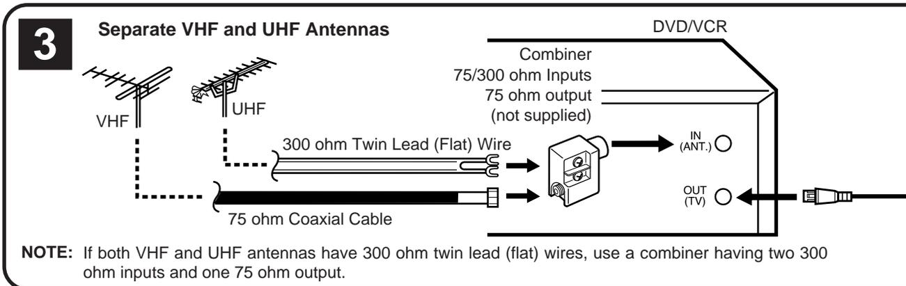
**NOTE:** If both VHF and UHF antennas have 300 ohm twin lead (flat) wires, use a combiner having two 300 ohm inputs and one 75 ohm output.
