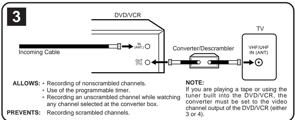
**NOTE:** Whenever a Converter/Descrambler box is placed before the DVD/VCR, you must tune the DVD/VCR to the output of the Converter/Descrambler box, usually channel 3 or 4.
