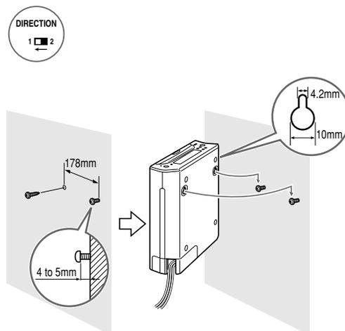
Mount two commercial screws onto the wall with each screw located in the same height.
