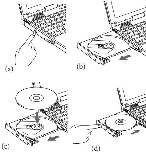
Figure 4-7 Loading/Ejecting Media
