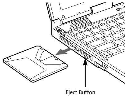
Figure 4-4 Loading/Ejecting a SuperDisk or 3.5" Floppy Disk
