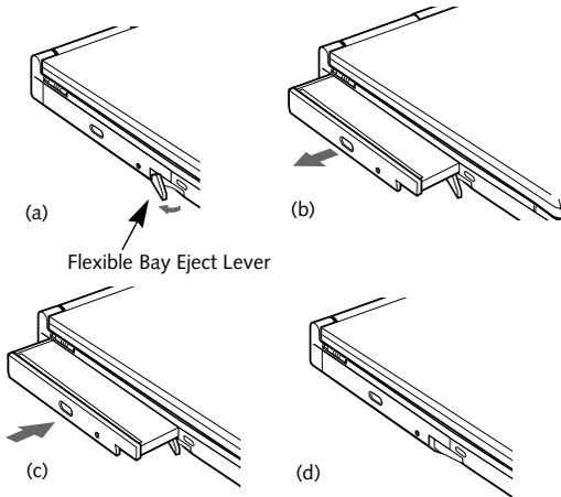
Figure 2-21 Removing/Installing a device in the Flexible Bay
