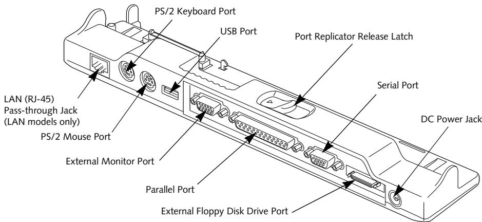
Figure 4-12 Port Replicator back panel (LAN model)
