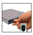
Connect the cable of the power supply to the Freecom Mobile DVD RW Recorder and the power supply itself to the socket.
