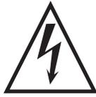
A triangle with a lightning symbol draws the user's attention to “dangerous voltage” without insulation in the housing which may be high enough to entail a risk of electric shock.
