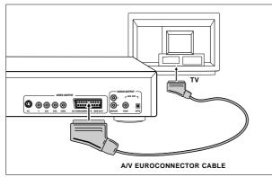
Connection to a TV with an A/V Euroconnector socket
