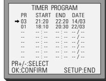
**2** Select the programming to change or erase. If you want to erase this programming press button [0], confirm with OK. If you wish to make changes: Move to the position you want to change using the [<, >] buttons. Change the settings using the [PR +/-] or [number] buttons. If all settings are ok, press [< or >], until you see "OK: CONFIRM" in the bottom line. Confirm changes with [OK]. Exit the menus.
