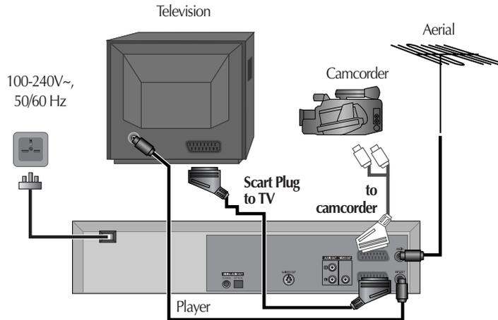
If you have connected your camcorder in this way, you can also connect a scart lead from "AV2" on the back panel of the player to the television. To use this function, see page 22.
