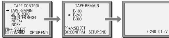
When you want the player to show the time remaining from the current player tape position (to find out if there is sufficient space for a recording, for example). To ensure the remaining time shown is accurate, select the length of cassette currently loaded by selecting this function until you reach the correct length.
