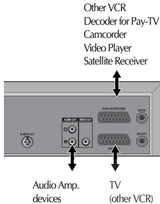
To copy to your player from another video machine, connect the two machines with a cable between their EURO AV (SCART) sockets and select as programme "AV 1/AV 2" or "F. AV" (front sockets) using the [AV], [PR+/-] or [ ] button.
