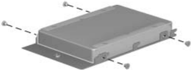
Figure C-11. PM3.0 × 3.0 Screw Locations
