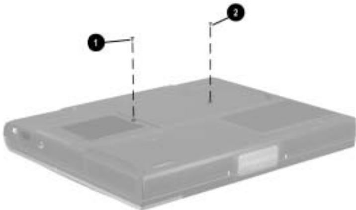
Figure C-12. PM2.5 × 4.0 Screw Locations
