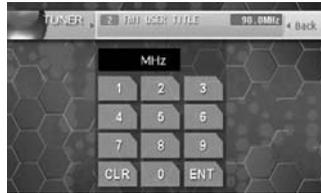
3. Touch the [0] to [9] key corresponding with the frequency you desired. When you input the wrong number, touch the [CLR] key to delete the last input number.
