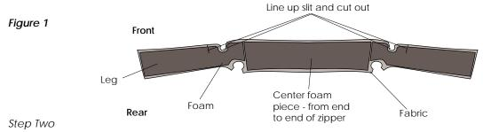
Determine the right and left leg foam. Line up the slit and the cutout in the foam with the seat belt cutout tab, and cutout in the fabric. Remove the protective strip from the back of the foam and press the adhesive strip on the foam to the fabric.
