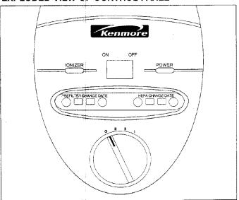
POWER CONTROL SWITCH and INDICATOR LIGHT - This switch will turn the air cleaner ON or OFF and has three speed selections: III (super), II (high) and I (low).
