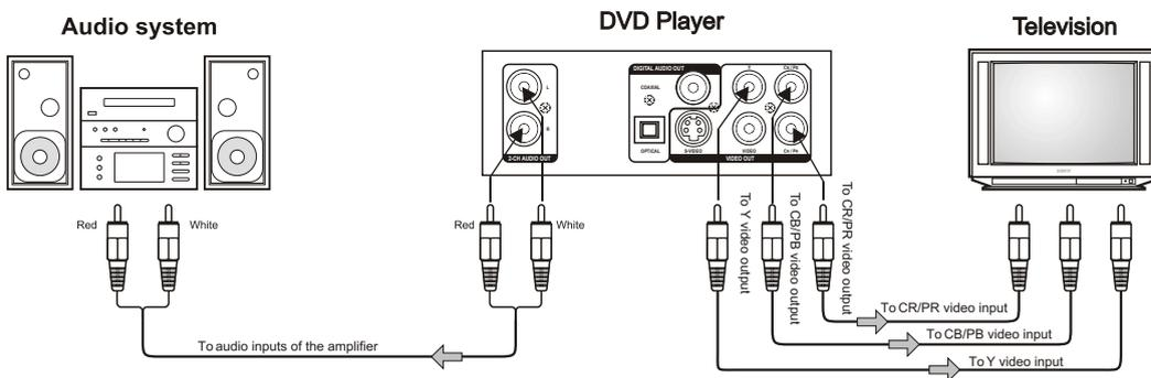
● **Connecting to an amplifier equipped with a digital audio input and TV**
