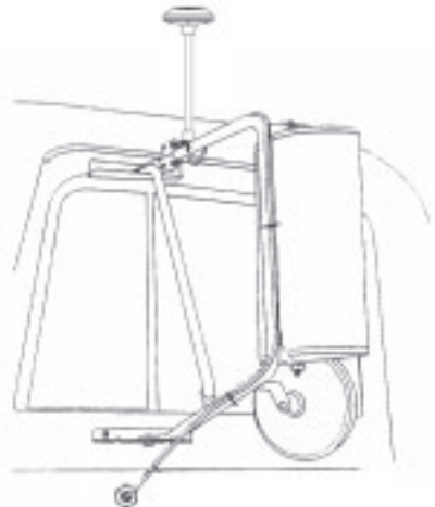
Figure 5. Mirror Mount Cable Routing
