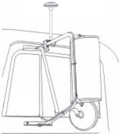
Figure 4. Mirror Mount Cable Routing
