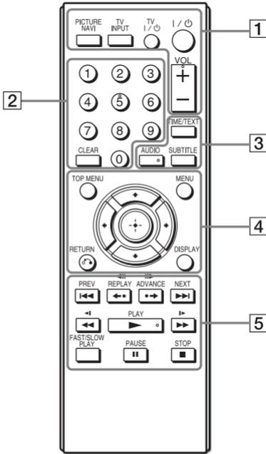
VOL +, number 5, AUDIO, and ► buttons have a tactile dot. Use the tactile dot as a reference when operating the player.
