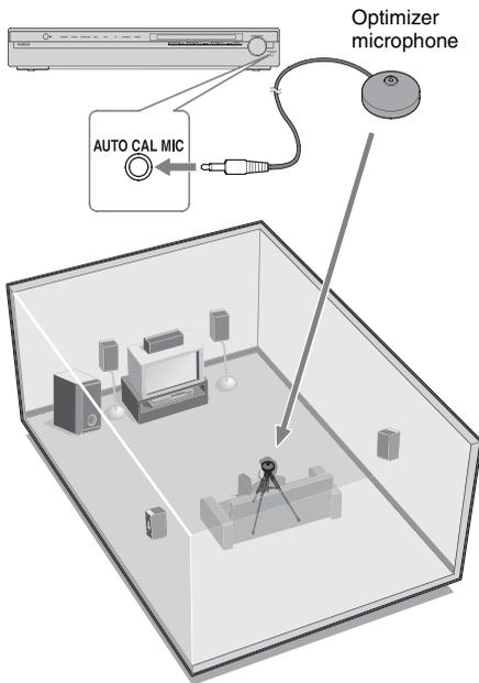
**1** Connect the supplied optimizer microphone to the **AUTO CAL MIC** jack on the front panel.
