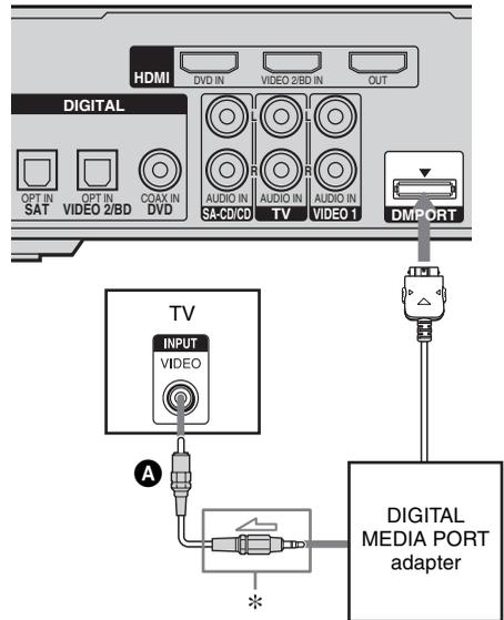
\* The type of connector varies depending on the DIGITAL MEDIA PORT adapter. For details, see the operating instructions supplied with the DIGITAL MEDIA PORT adapter.
