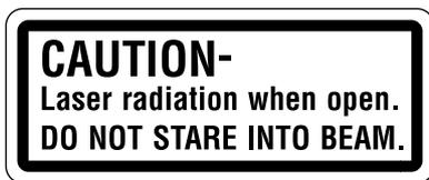
This label is located on the left side enclosure (Laser protective housing).
