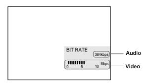
Bit rate refers to the amount of video/audio data per second in a disc. The higher the bit rate, the larger the amount of data. When the bit rate level is high, there is a large amount of data. However, this does not always mean that you can get higher quality pictures or sounds.
