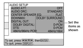
When you have made the connections using an optical or coaxial digital connecting cord, do not set "DOLBY DIGITAL" to "DOLBY DIGITAL," "DTS" to "DTS" and "48kHz/96kHz PCM" to "96kHz/24bit." If you do, a loud noise will suddenly come out from the speakers, affecting your ears or causing the speakers to be damaged.
