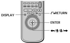
1 Press DISPLAY and select "SETUP" using ↑/↓.
