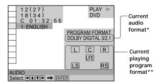
\* "PCM," "DTS" or "DOLBY DIGITAL" is displayed. In case of "DOLBY DIGITAL," the channels in the playing track are displayed by numbers as follows:
