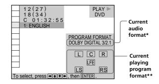
\* "PCM," "DTS," "DOLBY DIGITAL" or "MPEG" is displayed. In "DOLBY DIGITAL" case, the channels in the playing track are displayed by number as follows:
