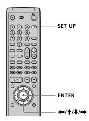
**1** Press SET UP to display the setup display on the TV screen.
