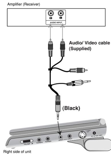
**Amplifier equipped with 2-channel analog stereo or Dolby Pro Logic II / Pro Logic:** Connect the AUDIO OUT jacks on the DVD player to the audio left and right IN jacks on your amplifier, receiver, or stereo system, using the audio cables.
