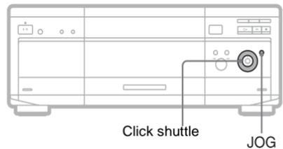
Turn the click shuttle on the player. The playback speed changes depending on the turning direction and degree of rotation as follows:
