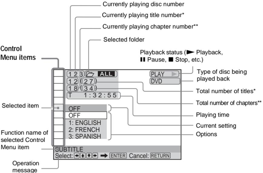
\* Displays the scene number for VIDEO CDs (PBC is on), track number for VIDEO CDs/CDs, album number for DATA CDs.
