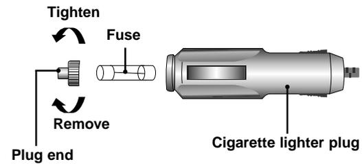
If this unit is not working properly, check to see if the fuse has blown out.
