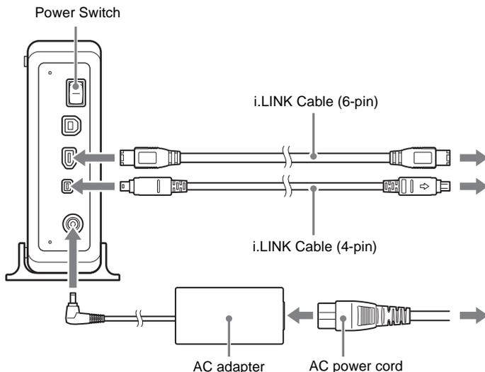
\* If your drive equipped with an AC IN connector instead of a DC IN connector, connect the provided AC power cord directly.
