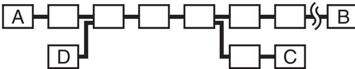
In any of paths A->B, A->C, A->D, B->C, B->D, and C->D, the maximum number of devices that can be connected is 17. (A maximum of 16 hops.)
