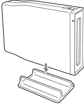
Position the drive so that the stand straddles the two anti-vibration pads on the drive bottom and then press it into place.
