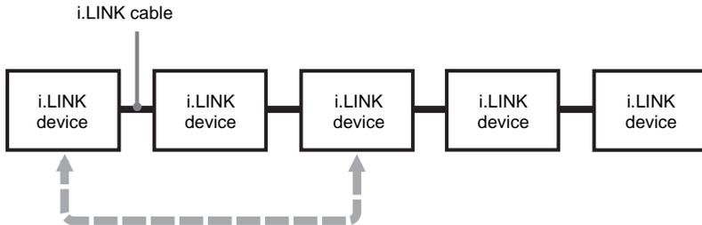
Data exchange and control are possible even when two i.LINK devices are connected through another device.
