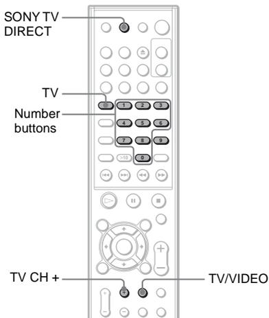
When you connect the
