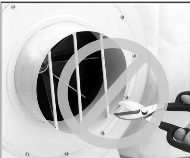
**Figure 5.** Do Not remove impeller guard.
