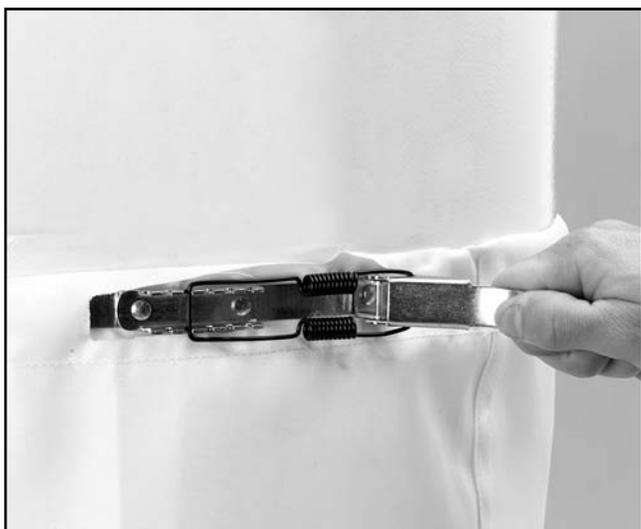
**Figure 15.** Securing the lower bag quick-release band clamp.
