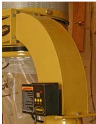
The smooth, flowing lines of this sheet metal chute make it very efficient. This chute replaces simple section of flex hose found on most dust collectors.
