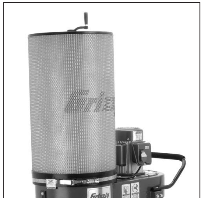
Figure 11. Canister filter installed and secured.
