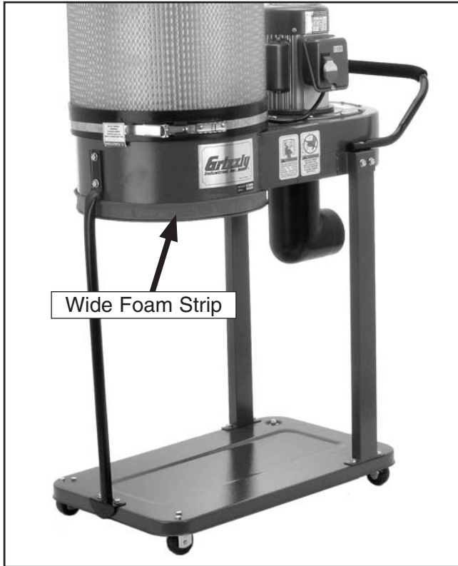
Figure 12. wide foam strip installed and trimmed.
