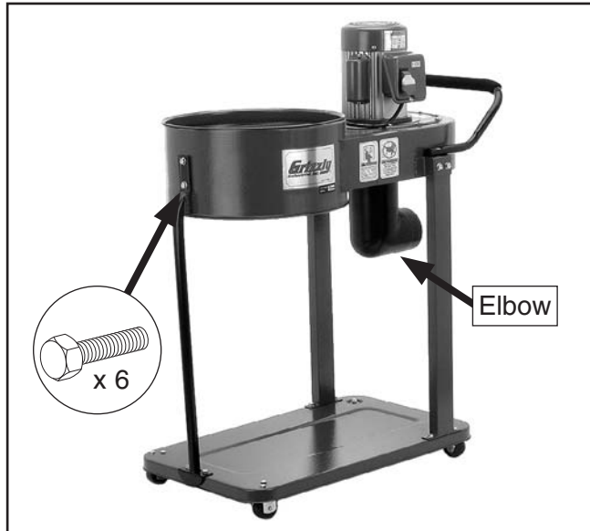
Figure 8. Impeller/separator attached to base.
