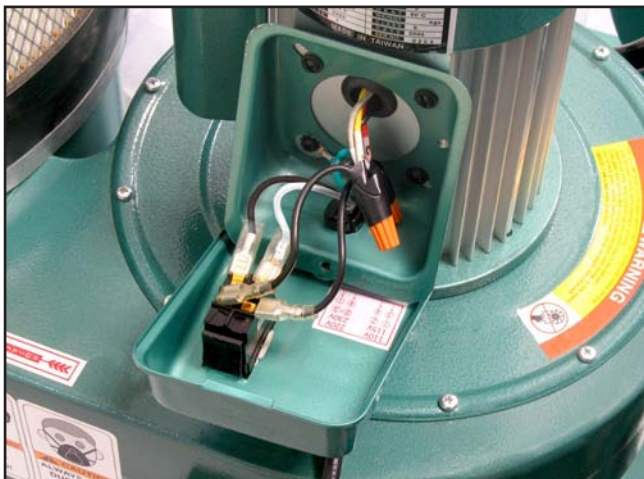
Figure 21. Motor junction box wiring.
