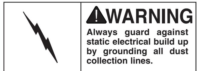
Be sure that you extend the bare copper wire down all branches of the system. Do not forget to connect the wires to each other with wire nuts when two branches meet at a “Y” or “T” connection.
