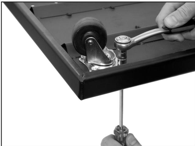
**Figure 5.** Installing casters.
