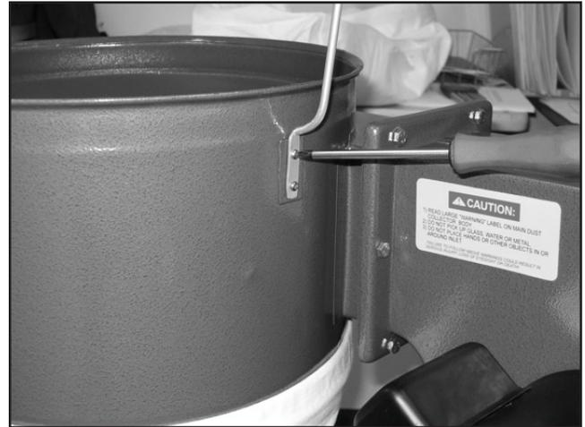
**Figure 10.** Installing upper bag support.
