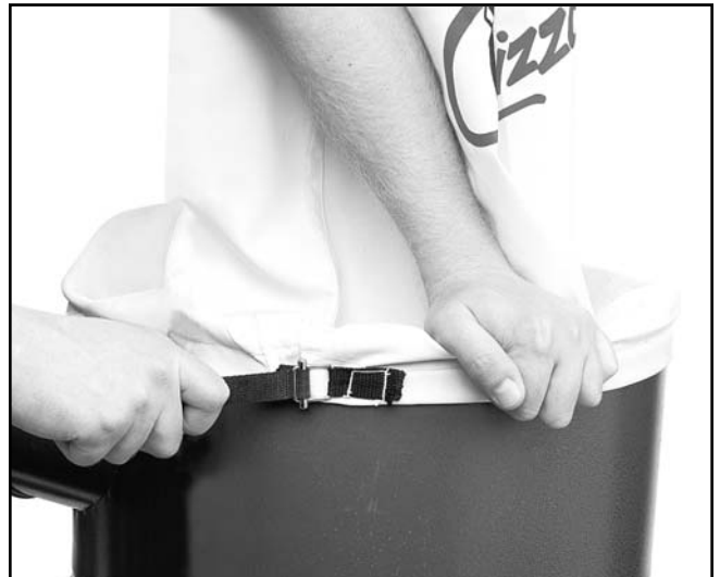
Figure 9. Securing collection bag.
