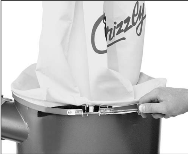
Figure 10. Tightening steel band.
