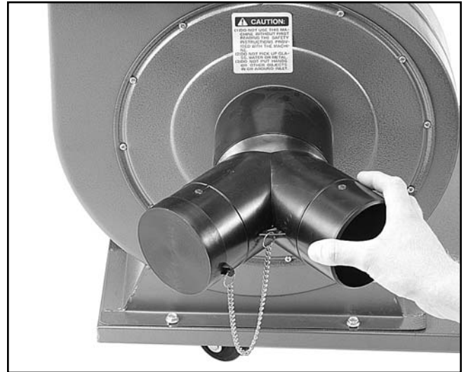
Figure 11. Installing “Y” inlet.
