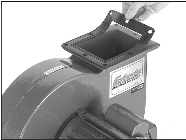
**Figure 9.** Placing rubber gasket over outlet.
