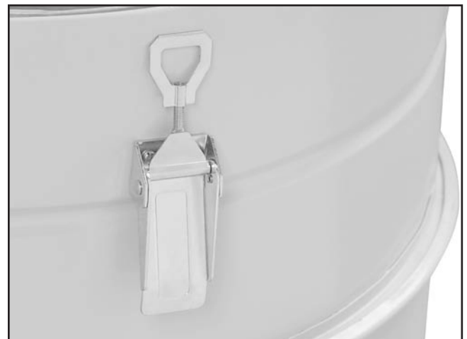
Figure 37. Collection drum lid latch installed.
