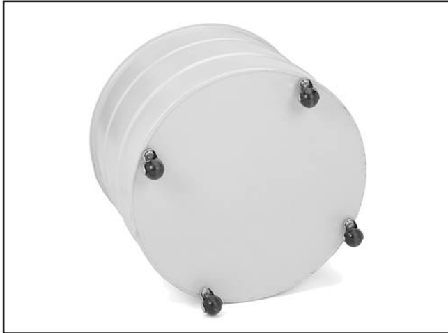
Figure 34. Dust collection drum casters installed.
