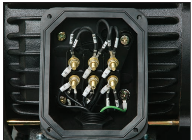
Figure 82. Model G0638 motor wiring (220V).
