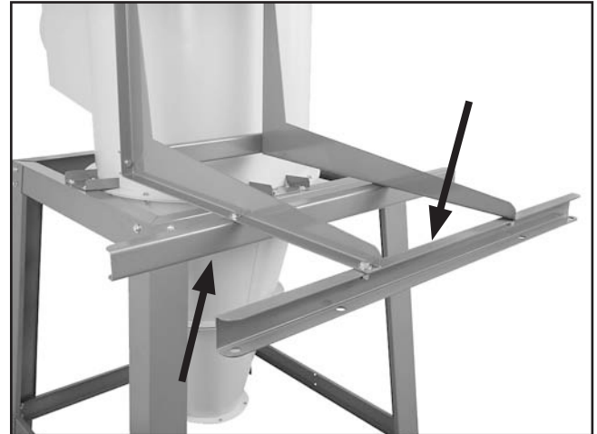
Figure 29. Long brace supports attached.
