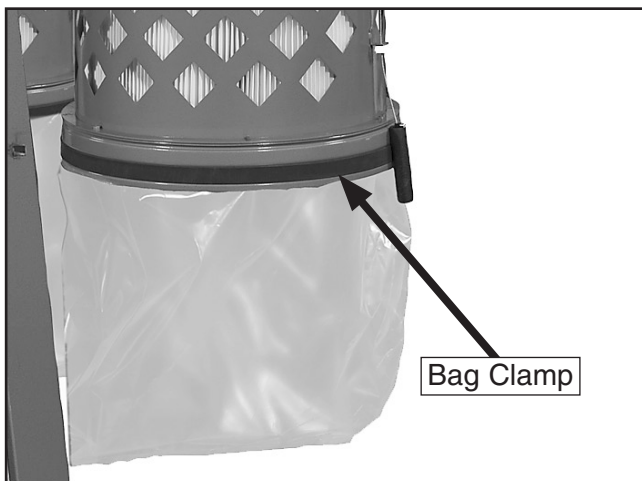
Figure 32. Canister filter collection bag installed.
