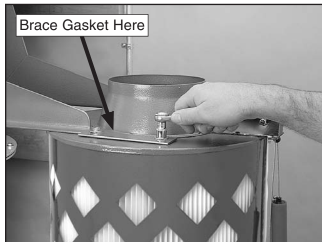
Figure 20. Mounting filters to the braces.
