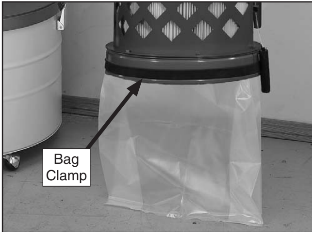
Figure 33. Plastic collection bag clamped in place under filter.
