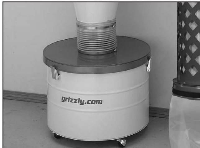
Figure 31. Drum attached to cyclone funnel with clear 9" hose.
