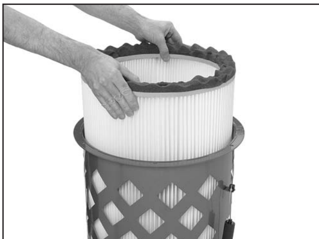
Figure 66. Removing the filter from the canister assembly.
