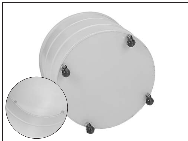
Figure 25. Casters attached to the lower collection drum.
