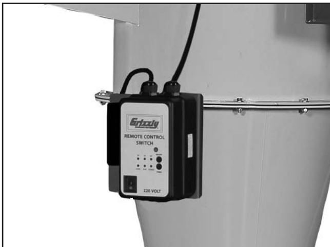
Figure 34. Switch mounted to funnel.
