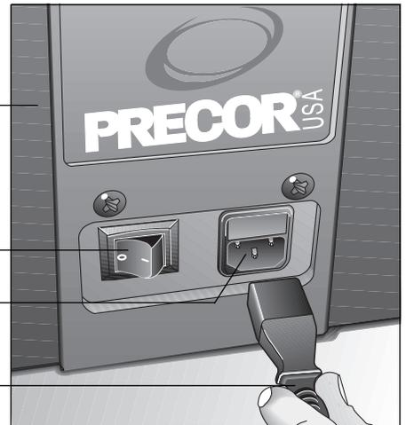
14. Plug one end of the power cord into the receptacle at the rear of the unit. See Diagram 7. Plug the other end into a standard 120v household outlet.
