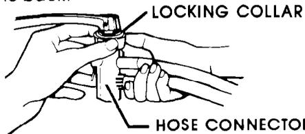
3. Pull down on the locking collar while lifting the hose connector onto the faucet adapter.
