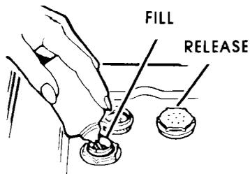
A rinse aid helps keep water from forming droplets and drying as spots. Keep the dispenser filled with a rinse aid such as Jet-Dry.<sup>®</sup> A small amount is released automatically during the final rinse of each cycle.
