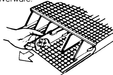
To remove the basket, slide it toward the top of the door – by the handle. Lift it off the holding buttons. Replace it in reverse order.
