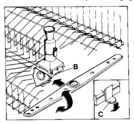
To do so, unhook the upper spray arm from the central support (B) by pressing the clip (C) and refit it in a reverse position (holes on the bottom). In this way the wash efficiency is improved, as the bottom basket is sprayed by both arms.
