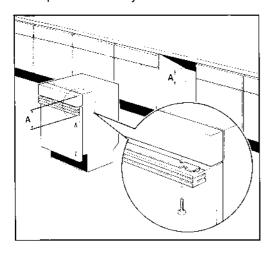
Measure the distance ("B") between the part below the control panel or fillets and the reference notch ("X") on the door.
