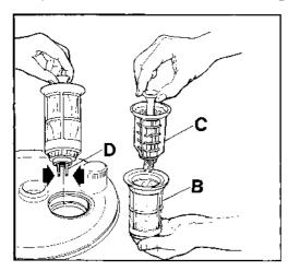
The filters (B and C) are both removed by lifting up the outer one (B) (pulling the central funnel upwards); the smaller filter (C) can then be removed by pressing the two tongues (D).
