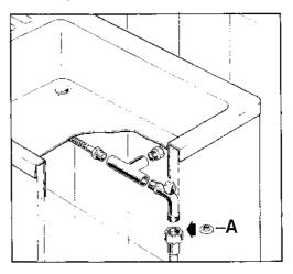
**Caution:** the retaining ring must be correctly fitted to avoid water leaks.
