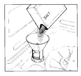
When this has been done, all you have to do is to periodically add salt to the container. You are reminded of this by the Salt refill light (7) on the control panel which illuminates when the salt has finished.
