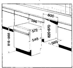
The recess ceiling may be anywhere between 820 and 870 mm from the floor inasmuch as the dishwasher incorporates levelling feet adjustable over a wide range (max 50 mm).
