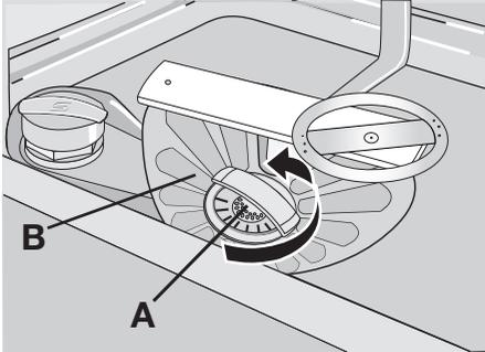
2. Filter (A) has two parts. To disassemble the filter, pull them apart.
