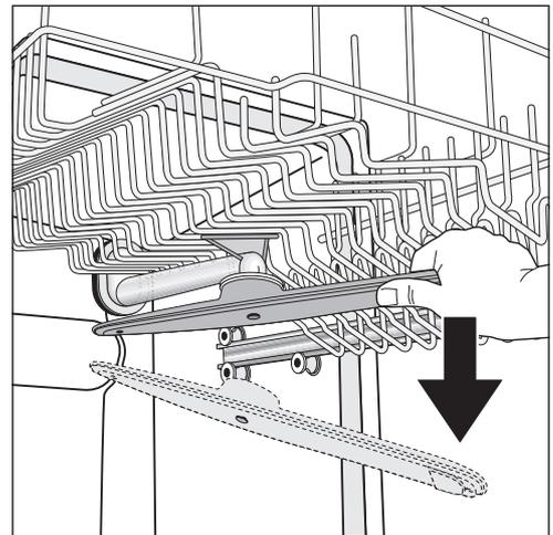
3. Place cleaned upper basket spray arm back in position against the connecting piece: press the two together firmly, until you feel them snap into place.
