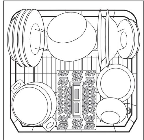
To make it easier to load larger dishes, the two rear plate rests in the lower basket can be folded down and the cutlery basket in the lower basket can be moved to the side.
