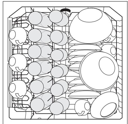
\*) If necessary, move the cup rack from right to left. When doing this, ensure that the cup rack is at the same height.
