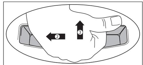
3. You can disengage the dishwasher's door safety catch by pressing the plate all the way to the left with your finger.
