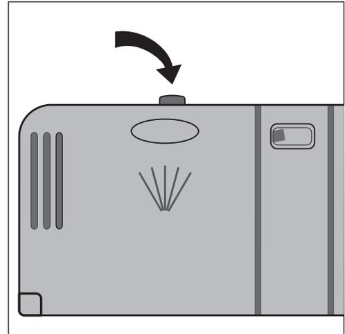
2. Place the detergent in the detergent dispenser. The markings indicate the dosing levels for powder detergents: "20/30" corresponds to approx. 20/30 ml of detergent. Follow the manufacturer's instructions with regard to dosing and storage.
