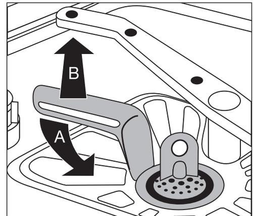
3. Grasp the grip hole on the fine filter (1) and remove it from the micro-filter (2).
