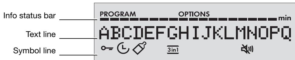
The **info status bar** consists of a row of individual lamps that is divided into two sections: the left section refers to the Programmes menu, the right section to the Options menu.
