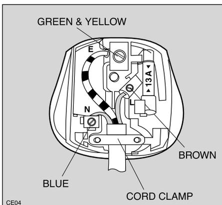
The plug moulded onto the lead incorporates a 13amp BS1362 fuse. Only ASTA or BSI fuses should be used.
