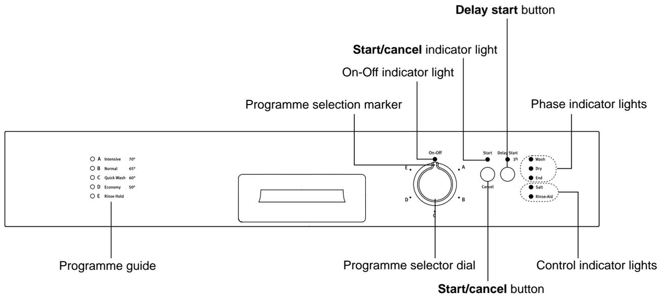
**Programme selector dial and On-Off indicator light:** the selection of a washing programme occurs by turning the programme selector dial clockwise or anticlockwise, until the desired washing programme (see "Washing programmes" chart) corresponds with the programme selection marker placed on the dial (position **On**). The On-Off indicator light illuminates. The indicator lights of the phases foreseen for the selected programme start flashing.
