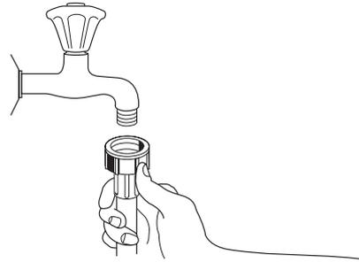
**!** Check that the nut and all other connections are tight before the machine is moved into position.
